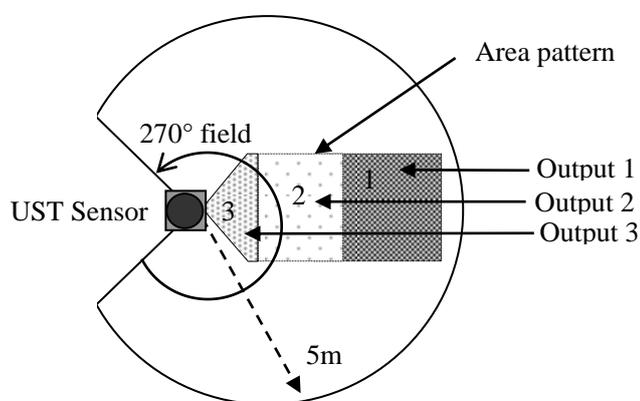
Figure. 1: Detection area and outputs in UST Sensor
